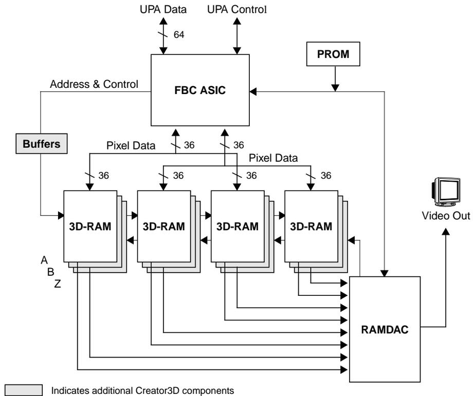
Figure 3-2 Combined Block diagram of Creator and Creator3D
