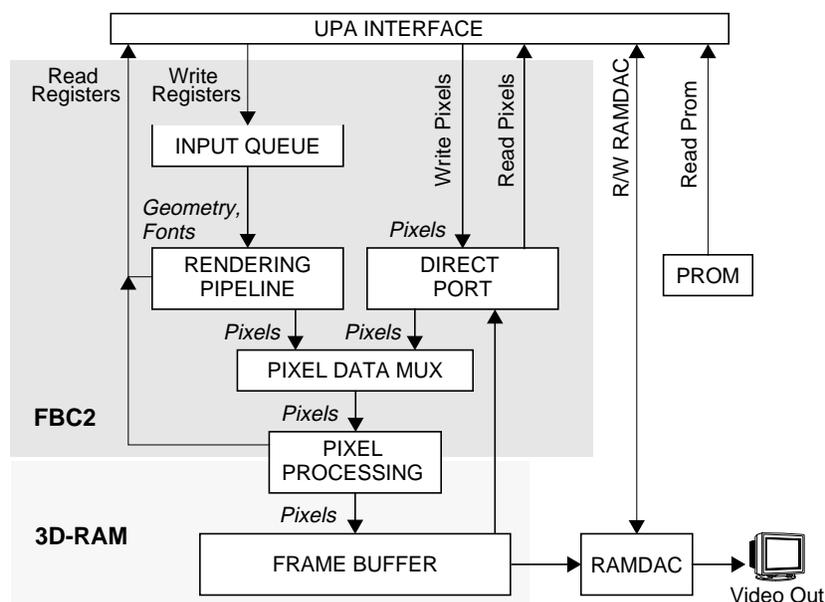
Figure 3-3 A logical view of the Creator Graphics subsystem
